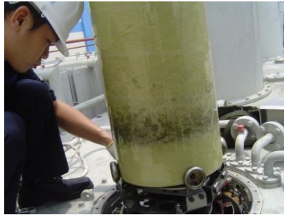
OLTC upon removal from its compartment. Due to long time operation, Transformer insulating cylinder was thickened with carbon residue from breakdown of insulation oil.
