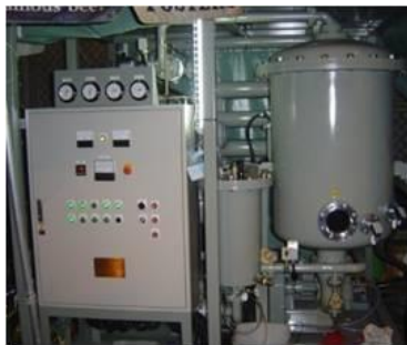
Oil filtration machine for oil treatment.
